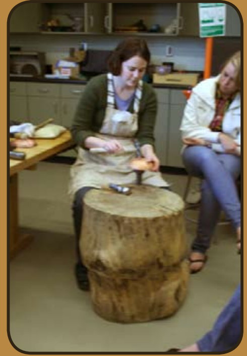
Corey Ackelmire demonstrates sinking a bowl. Here she is planishing the surface, which means smoothing out lumps with light blows from a polished hammer. Elizabeth Seward (right) is a senior at Riverside and a morning metals student at the FAC. Said another student, Jena Heaton, who watched the demonstration, "It was so cool to see how a flat sheet of metal became a more complex shape."
